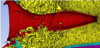
Figure 13 Copper cone of the SC after impact of a fragment.
