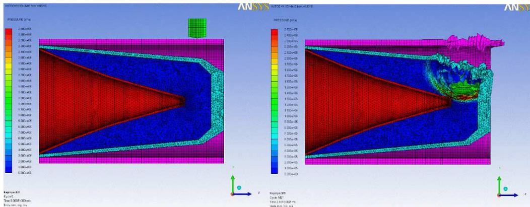
Figure 15 Fragment impact simulation with fragment impacting near the bulk of the explosive material.
