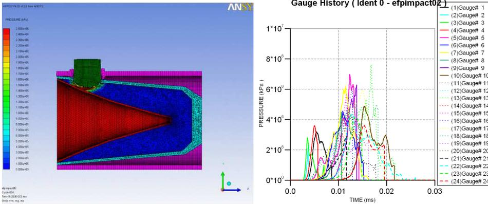
Figure 12 Result of the simulation of the short thick EFP (27mm) at a velocity of 2100 m/s.
