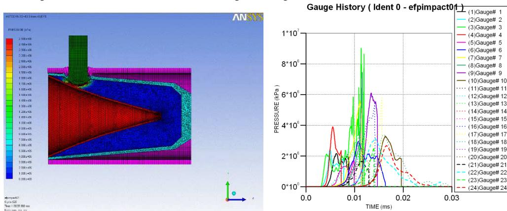
Figure 11 Results of the simulation with the long EFP (19 mm diameter).
