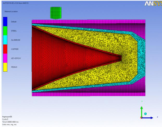
Figure 6 Grid and materials used for the simulation.
