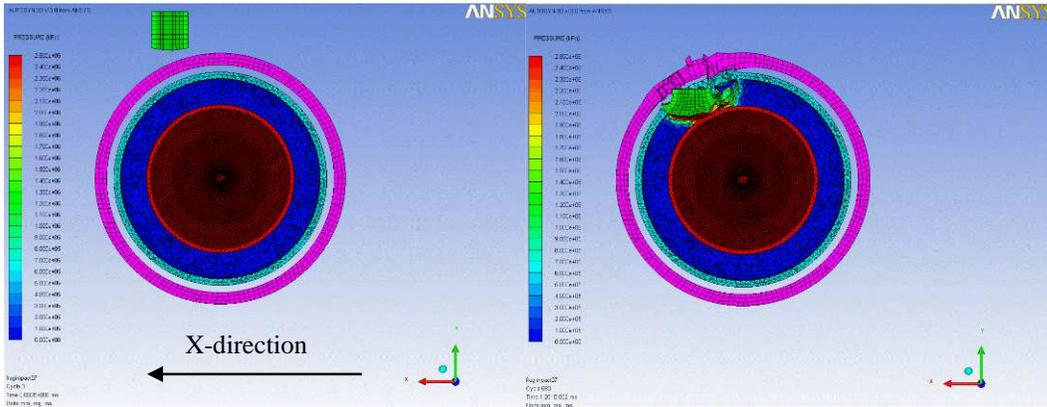
Figure 9 Cross-section pictures of the SC warhead in off-center impact scenario. On the left the location of impact on the right after penetratin the warhead.
