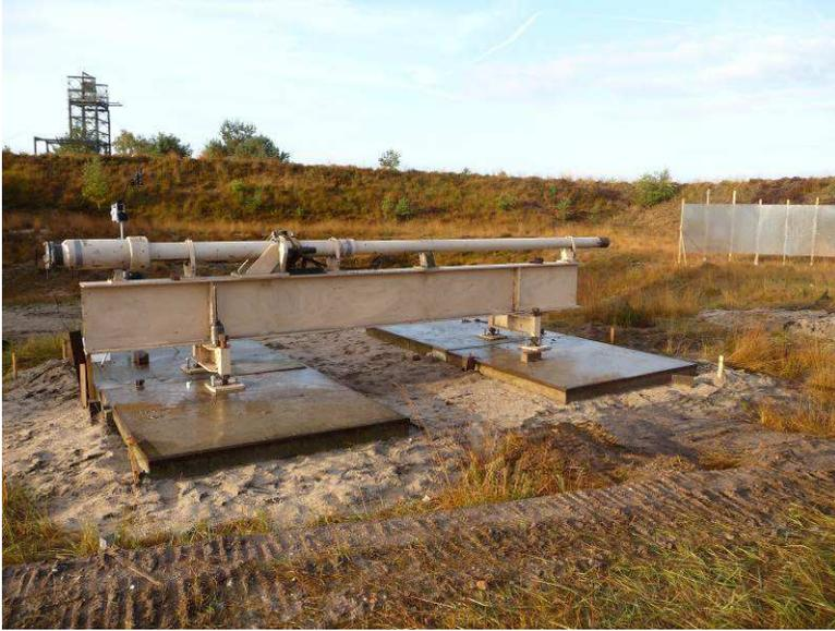
Figure 1 TNO's 50 mm gun for launching the standard IM fragment to a speed of 2530 m/s.
