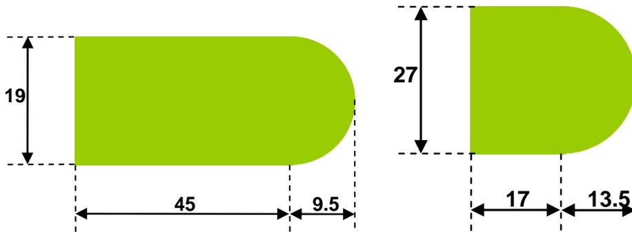
Figure 5 The characteristic parameters of the two basic EFP's.
