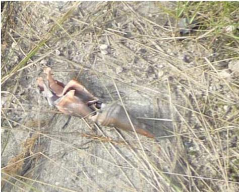
Figure 3 The shape of the copper liner after the reaction.
