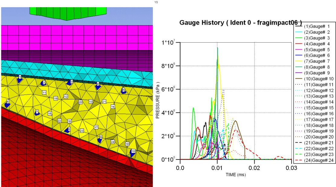
Figure 8 location of the gauges on the left and the corresponding pressure graphs as a function of the time on the right.
