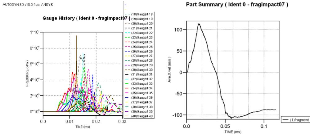
Figure 10 The pressure in the explosive with an off-centre impact location (left) and the velocity change in the x-direction (right).
