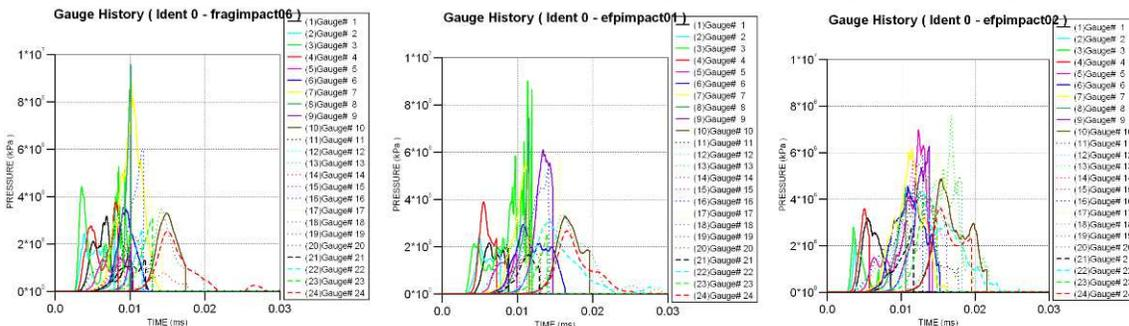
Figure 14 The shock pressures in the explosive due to the impact of the projectiles; fragment impact at 2530 m/s left, 19 mm EFP at 2100 m/s middle and the 27 mm EFP at 2100 m/s on the right.
