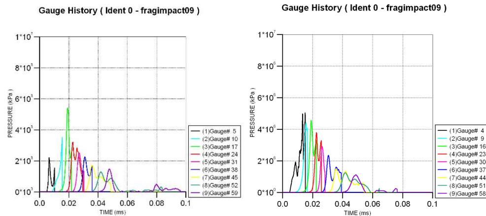
Figure 16 Pressures during the impact around the bulk of the explosives.
