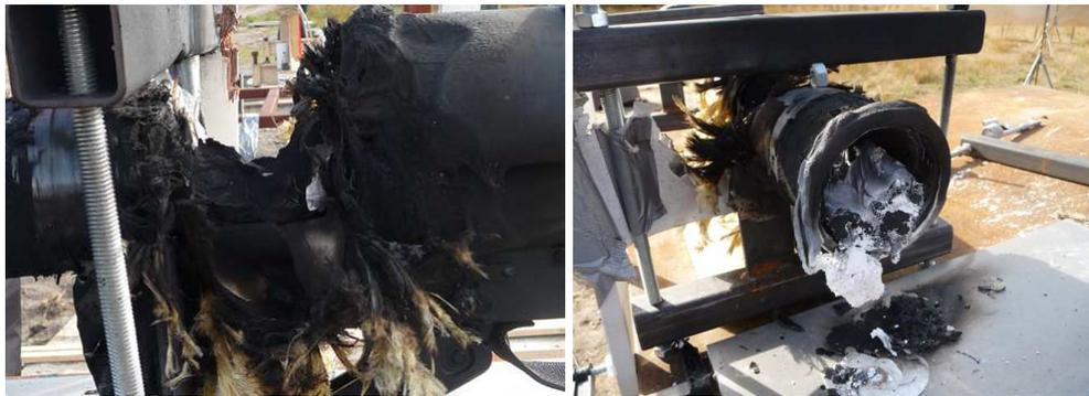
Figure 2 Burning of the Shaped charge warhead after being hit with a fragment.
