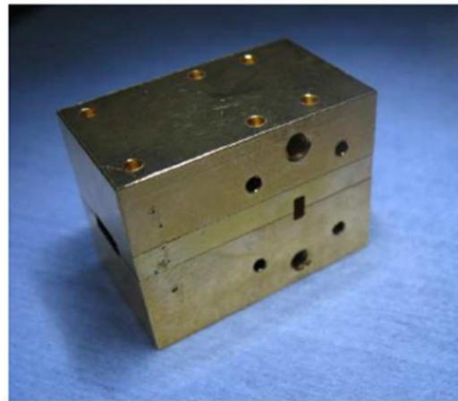
Fig. 11: Single chip waveguide module showing the mounted MHEMT power amplifier MMIC.
