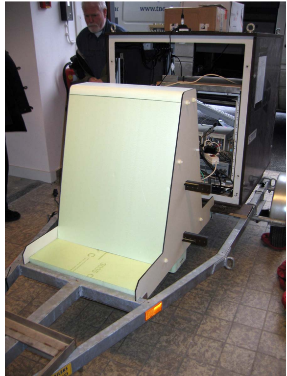
Fig. 3 Antenna system of the radar mounted at the TNO test platform
