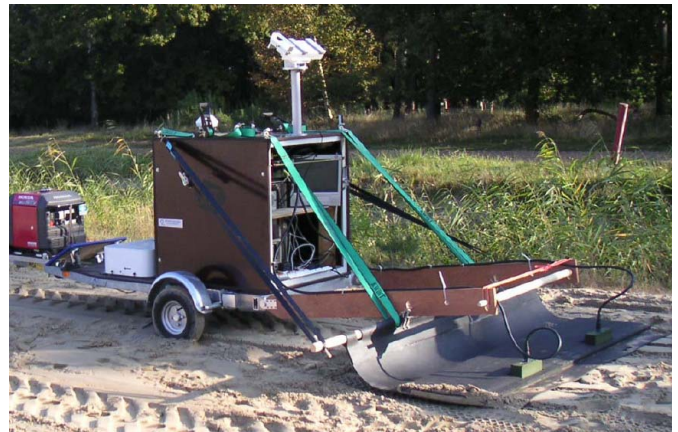
Fig. 1. TNO multi-sensor test trolley for landmine detection research
