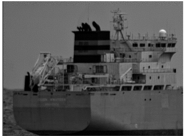
Figure 4. Originally recorded maritime visible light image (top) and image processed with turbulence corrector (bottom). The ship's range is 12.5 km. Images were recorded with the TNO SPITS [2] system.
