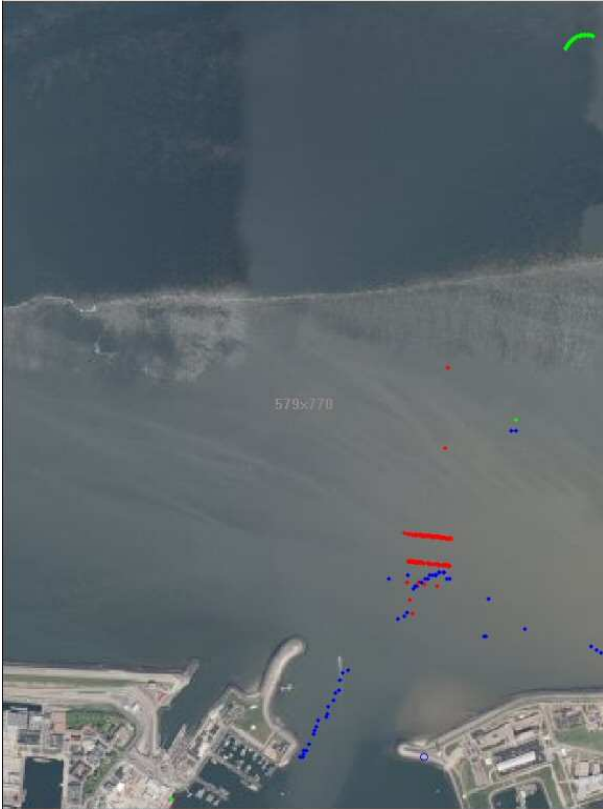
Figure 13. This sensor data fusion harbour scenario contains a patrol boat, RHIB and other opportunity vessels. Radar tracks (in blue) and infrared tracks (in red) (with green GPS/AIS).
