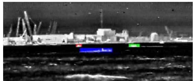
Figure 14. Classified objects during a real-time trial in the Rotterdam harbour. The automatically classified targets are coloured: watertaxi (red), RHIB (green) jet-ski (blue).
