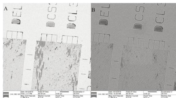
Figure 2: a) HIM image of old reticle before and b) after first 1 hour cleaning step
