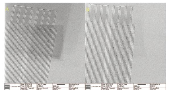
Figure 5: a) HIM image of SEM deposited carbon and b) the same image after 10 min plasma treatment
