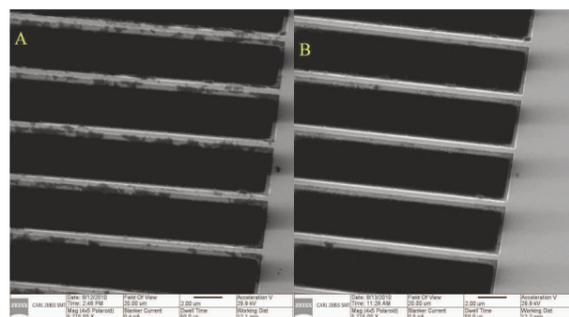
Figure 3: a) HIM image of single lines and spaces before and b) after first 1 hour cleaning step
