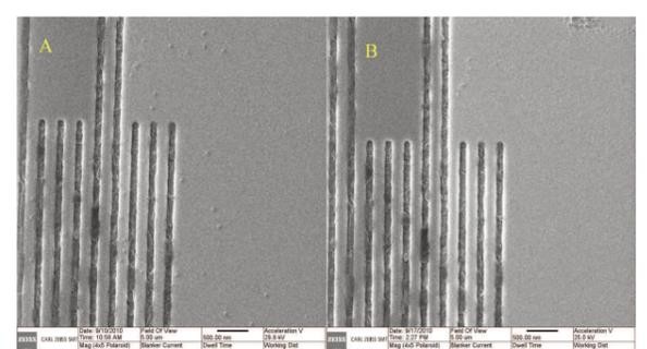
Figure 6: a) HIM image of reticle with 50 nm PSL spheres before and b) after 10 min plasma treatment
