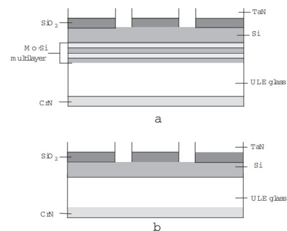
Figure 1: schematic layout of dummy reticle
