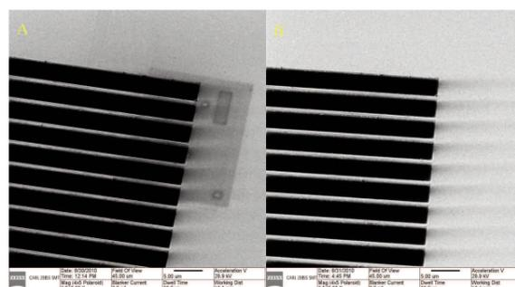
Figure 4: a) HIM image of single lines and spaces before and b) after first 10 min of cleaning
