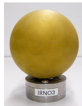
Fig. 2. Artefact: ball ( \text{\O} = 120.0159 mm, sphericity = 22.1 \mu\text{m} )
