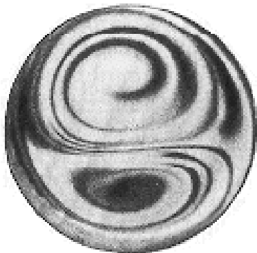
Figure 2. Dean vortices moving from the wall to the centre of the tube and vice versa
