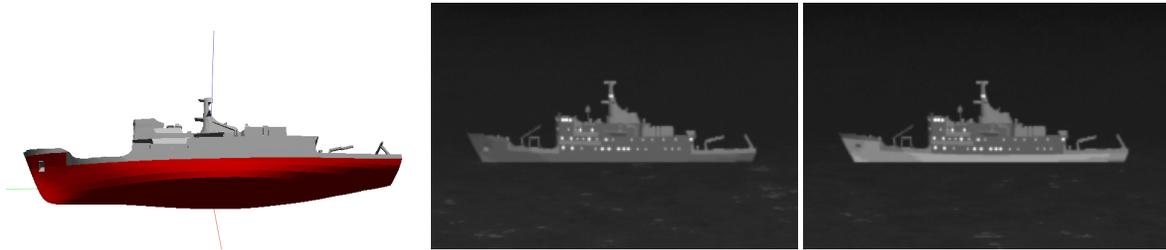
Figure 10: Effect of forced temperature changes in ship signature modelling. The left panel indicates the part of the ship in red where the temperature is replaced by a higher temperature. The middle panel shows the ship signature in equilibrium and the right panel shows the effect of an increased hull temperature.
