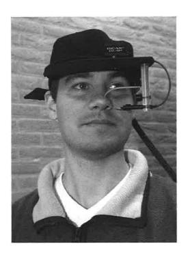
Figure 10.1 The ISCAN eye movement equipment that was used during the experiment with the apparatus being attached to a baseball cap.
