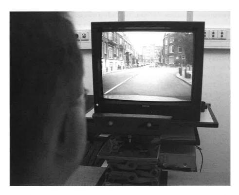
**Figure 12.5** A participant watching the video. The Tobii equipment is visible just below the television monitor with the two dots being the infrared light sources.
