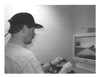
Figure 9.1 The task environment of the experiment, with a participant driving through the virtual environment, wearing the eye movement equipment.
