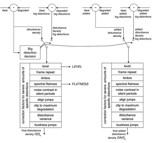
Fig. 3. Overview of the second part of the POLQA perceptual model. Calculation of the final disturbance densities from the four different variants of the internal representations distortions (see Sections 2.11 and 2.12).
