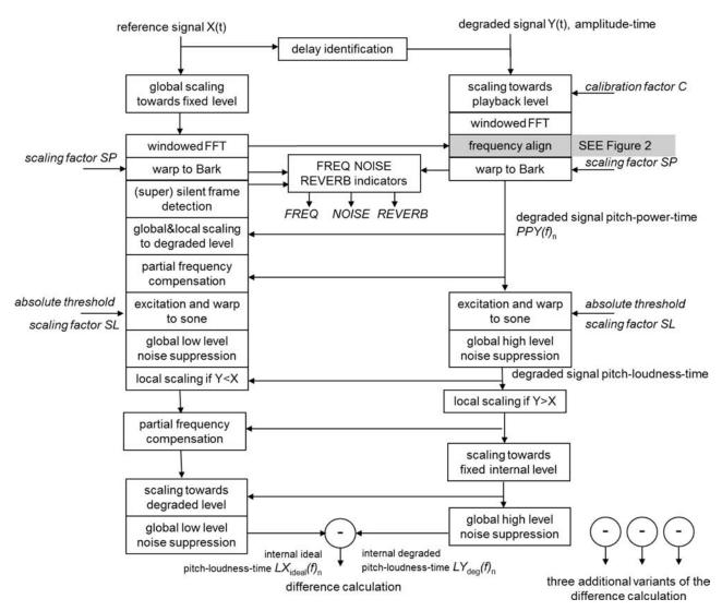
Fig. 1. Overview of the first part of the POLQA perceptual model: Calculation of the internal representation of the reference and degraded signals (see Sections 5.1 through 5.10). Four different variants of the internal representations are calculated (represented by the four circles with a - sign), each focused on a specific set of distortions (see Sections 2.11 and 2.12).
