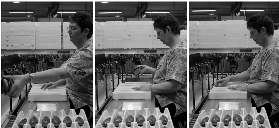
Figure 2-2. Detailed view of the assembly task in case study 2. Picking the product (left), visual control (middle) and placing the product (right).
