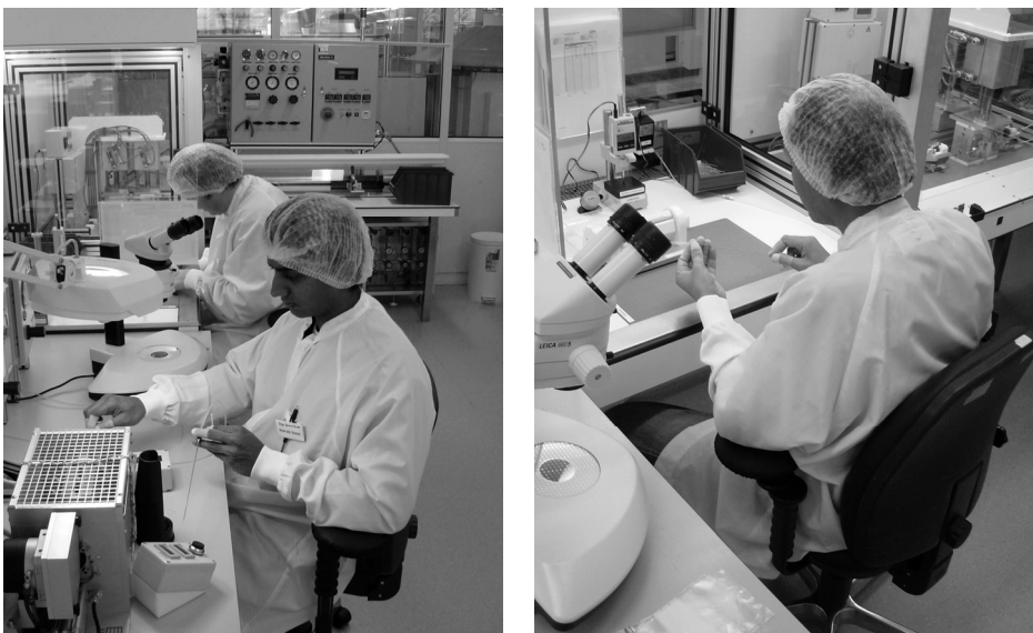
Figure 2-1. A double workstation for the assembly of catheters (left). A detailed view of the production of catheters in case study 1 (right).
