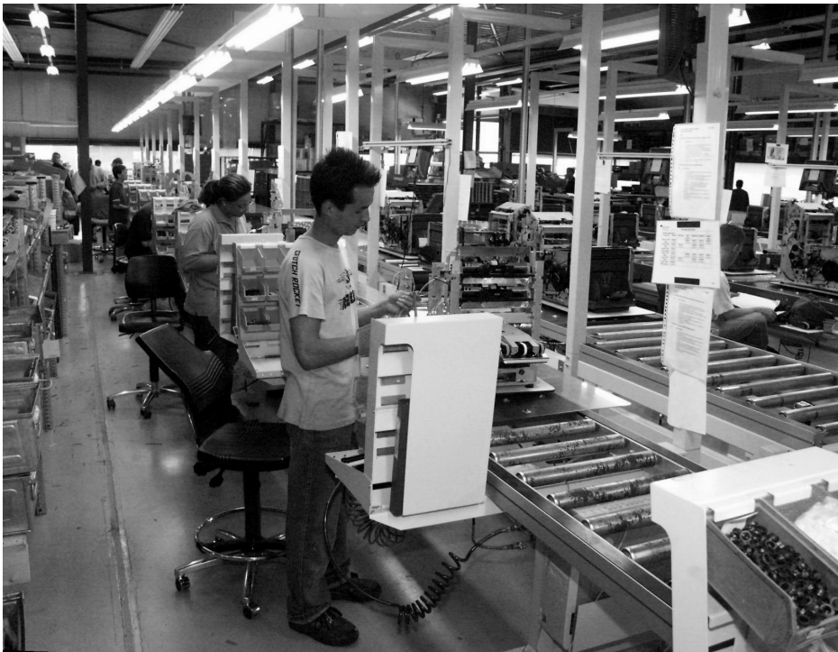
Figure 8-1. Work station design can stimulate variation in workload and thereby reduce fatigue and stimulate performance. Decentralizing bin locations of product specific components force operators to change working posture.
