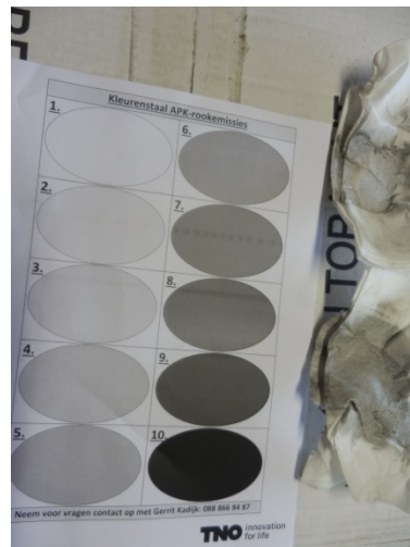
Figure 3: Tissue mounted on a tail pipe for a smoke emission test.
