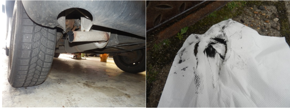
Figure 1: Tailpipe and result of inner tailpipe test
