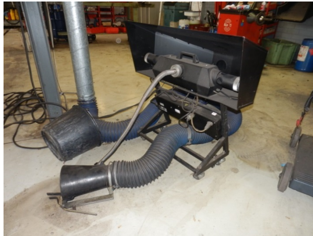
Figure 5: Opacity meter for a roadworthiness test.
