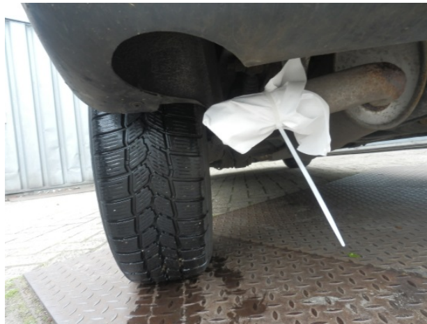
Figure 3: Tissue mounted on a tail pipe for a smoke emission test.
