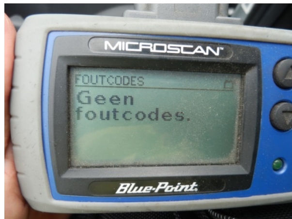
Figure 2: EOBD reader, displaying the message "No error codes".
