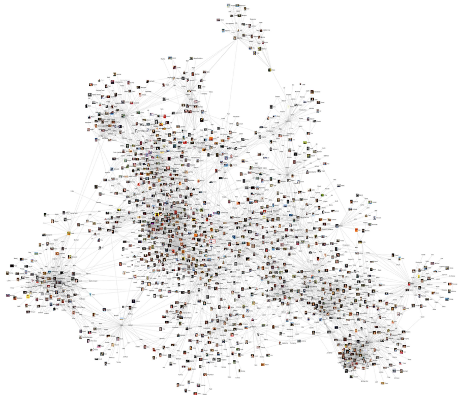
Figure 8 Force-based or force-directed or Spring-embedder layout. This is a class of algorithms that assign forces as if the edges were springs (Hooke's law) and the nodes were electrically charged particles (Coulomb's law). The entire graph is then simulated as if it were a physical system. This results in highly connected individuals migrating to the center, while less connected individuals are pushed to the outside. Most tools use the Fruchterman-Reingold algorithm in combination with the Kamada-Kawai algorithm. It often gives aesthetically-pleasing layouts, but the algorithms have slow run time, it can take quite a while before the network 'settles', i.e. reaches equilibrium. Image from [Heer05].
