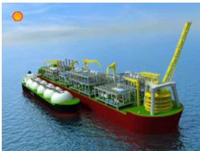
Figure 2.1. A picture of the Shell Prelude Floating LNG factory, that will be built in the next 4 years. The ship will be 488 m x 74 m.
