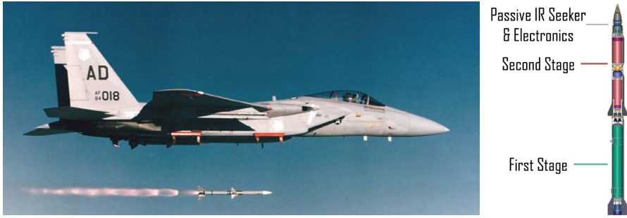
FIGURE 3.17: AMRAAM fired from F-15 [81] and breakdown of the NCADE AMRAAM [80].
