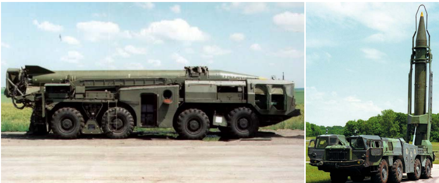
FIGURE 2.7: Transporter-Erector-Launcher (TEL) loaded with a TBM (Scud) [18].
