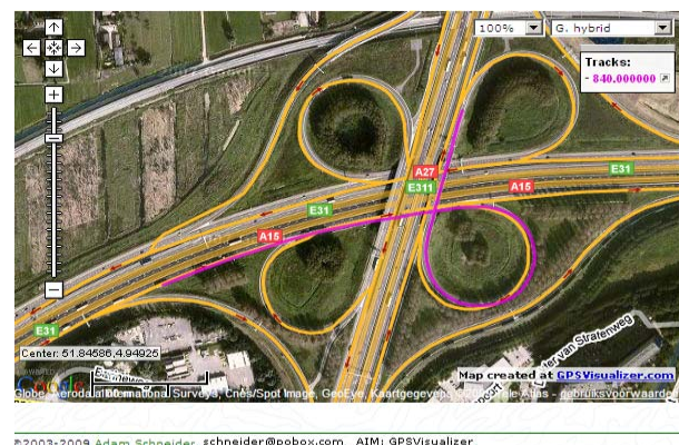
Figure 7. Cloverleaf with highest measured level of roll over risk and DC intervention.
