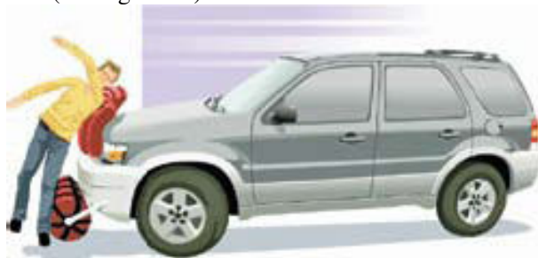
Figure 19 - Autoliv airbags concept for a SUV. Front edge and bumper airbag
