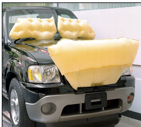
Figure 21 - Ford airbag system
