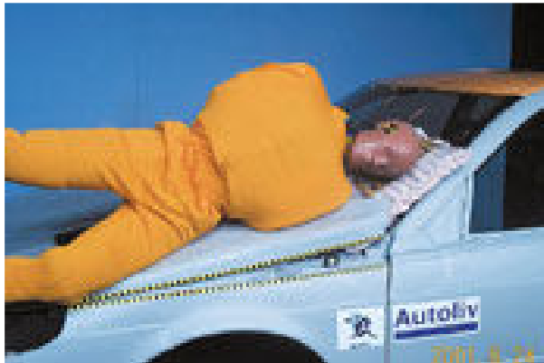
Figure 20 - Autoliv A-pillar airbag.
