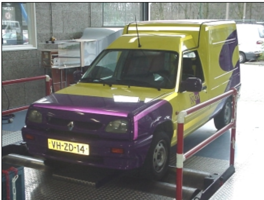
Figure 41: Renault Express Electrique on the IAE dynamometer
