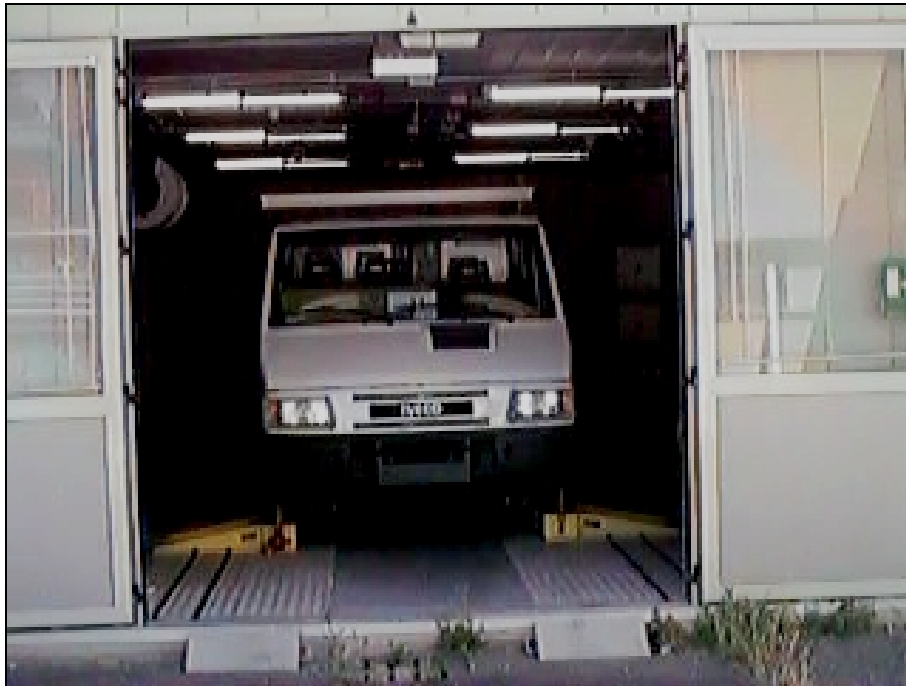
Figure 30: ALTROBUS on the ENEA dynamic rollerbench
