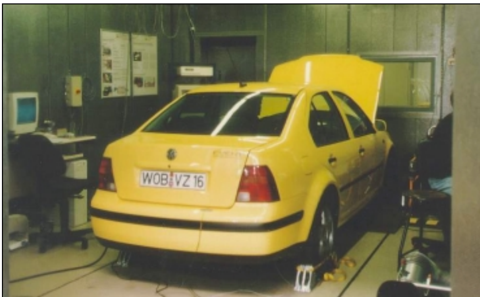
Figure 3.1-1: Volkswagen Bora electric vehicle on the dynamic rollerbench of the ika
