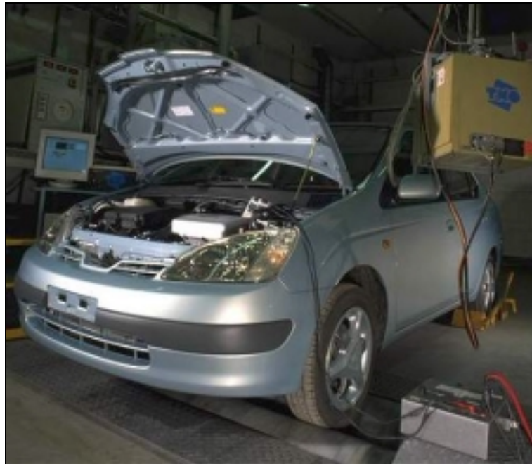
Figure 9: Toyota Prius on the rollerbench at TNO
