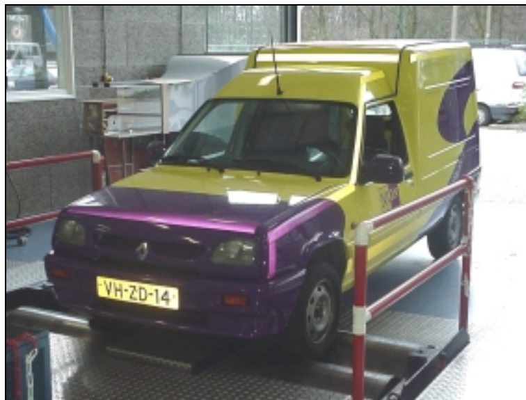
Figure 27: Renault Express Electric on the IAE dynamometer
