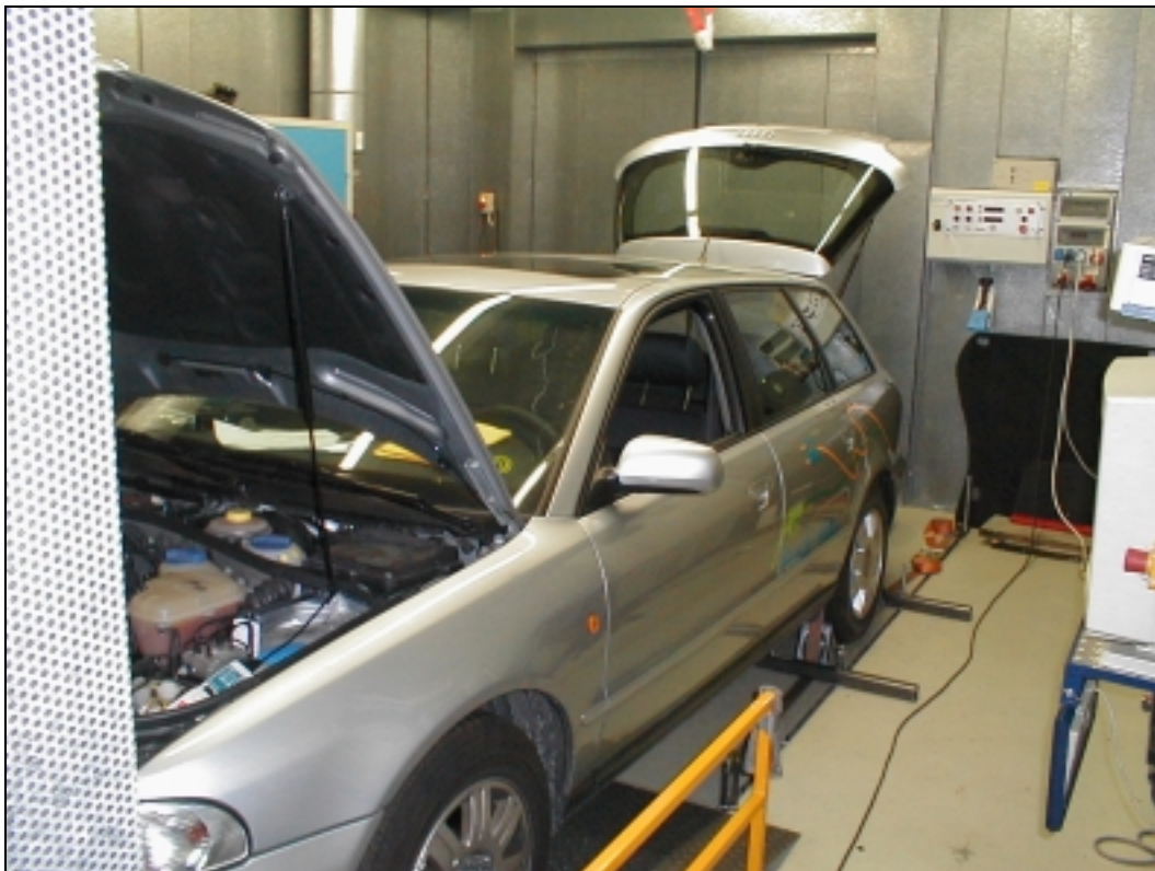
Figure 3.2-1: Audi Duo on the dynamic roller testbench of the ika
