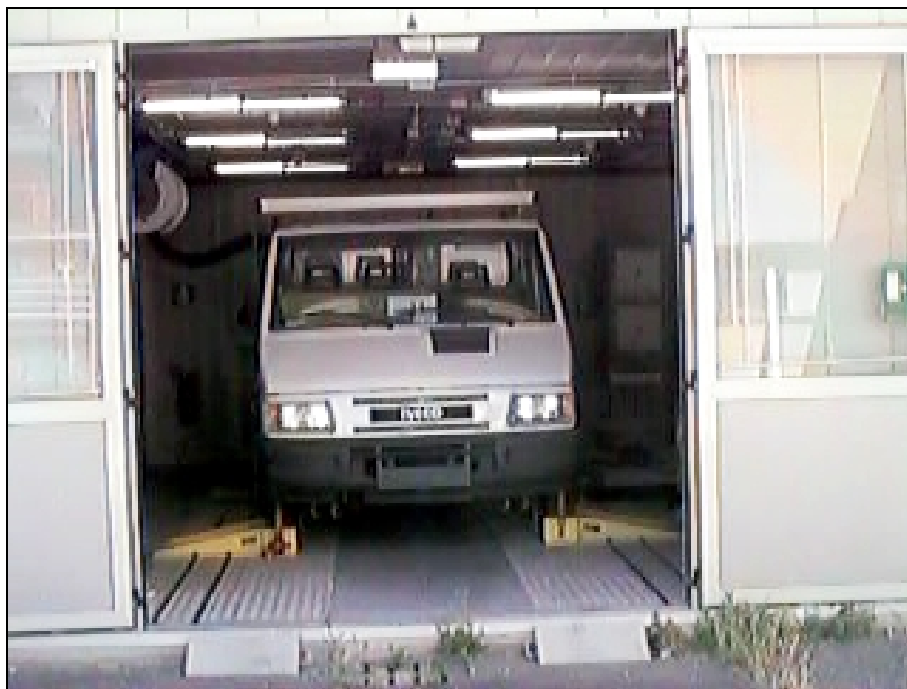
Figure 16: The ALTROBUS on the dynamic rollerbench at ENEA, Italy
