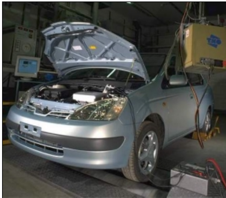
Figure 23: Toyota Prius on the rollerbench at TNO
