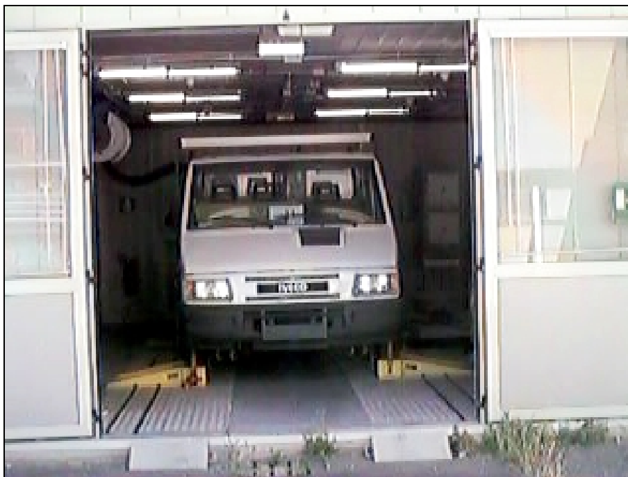
Figure 42: ALTROBUS on the ENEA dynamic rollerbench
