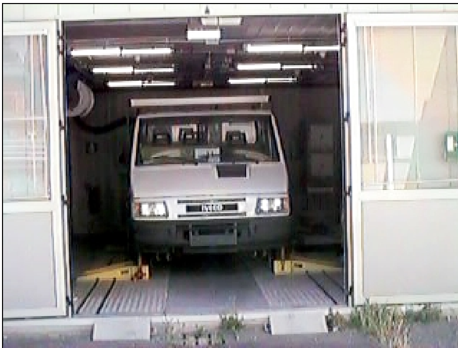
Figure 61: ALTROBUS on the ENEA dynamic rollerbench
