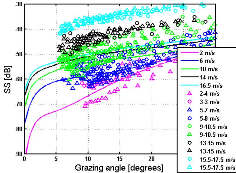
Fig. 4. Theoretical (curves) total backscattering predictions at 940 Hz based on the HN model compared to surface back-scattering measurements (symbols) obtained during the Critical Sea Test Experiments [4]. The legend indicates the wind speed values ( $v_{10}$ ).
