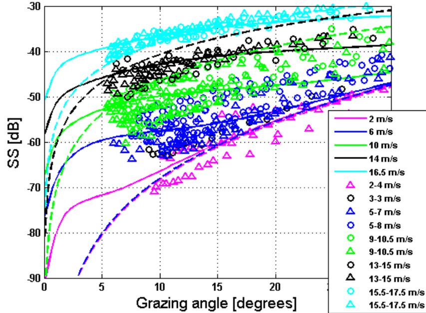
Fig. 6. Theoretical (solid curves) total backscattering predictions at 940 Hz based on the extended HN (including bubbles larger than 1 mm) model compared to surface backscattering measurements (symbols) obtained during the Critical Sea Test Experiments [4]. The legend indicates the wind speed values ( $v_{10}$ ). The dashed lines are the empirical Ogden-Erskine predictions for the same conditions as the solid lines.
