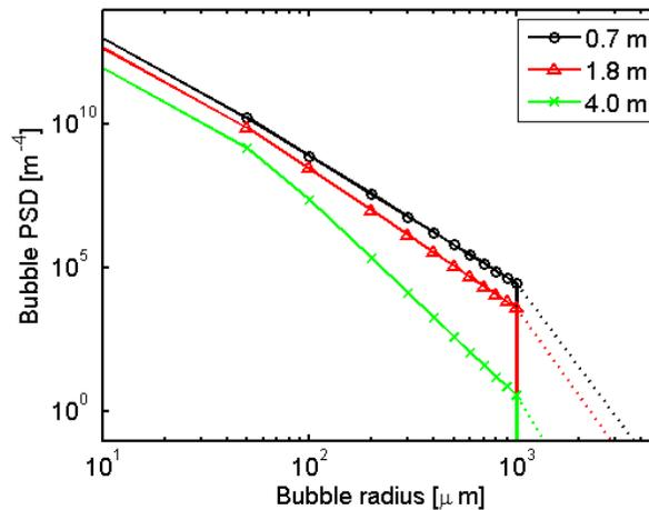
Fig. 3. Hall-Novarini bubble population spectral densities for a wind speed ( $v_{10}$ ) of 14 m/s (solid). The dashed curves show the extrapolation of the Hall-Novarini model for large bubbles. The curves correspond to 0.7, 1.8 and 4.0 m depth, respectively.
