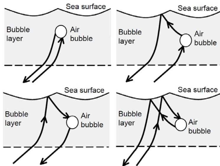
Fig. 2. The four different volume scattering contributions for a single bubble.
