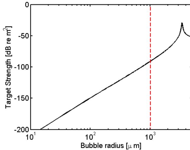
Fig. 5. Bubble target strength as a function of radius at 940 Hz. The red line indicates the separation between the bubbles that are included in the HN model and the extended HN model.
