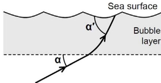
Fig. 1. The effect of a near-surface bubble layer on the grazing angle
