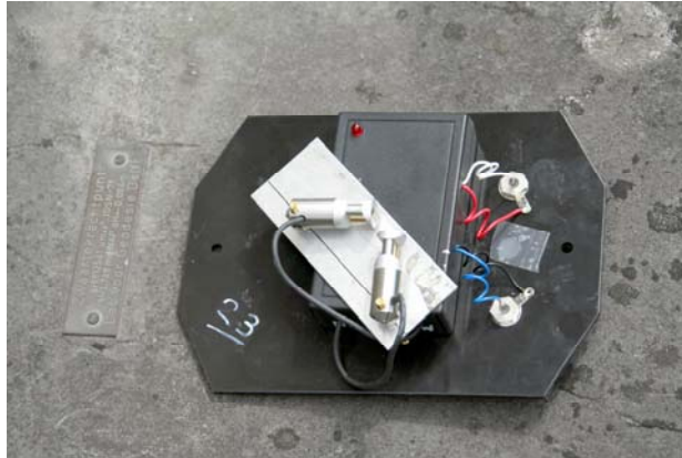
Fig. 1: A photograph of a measurement station. The Microflown probes are oriented perpendicular and are mounted on the electronic box. The coloured wires lead to the connectors for the signal cables. A probe is 1/2 inch wide.
