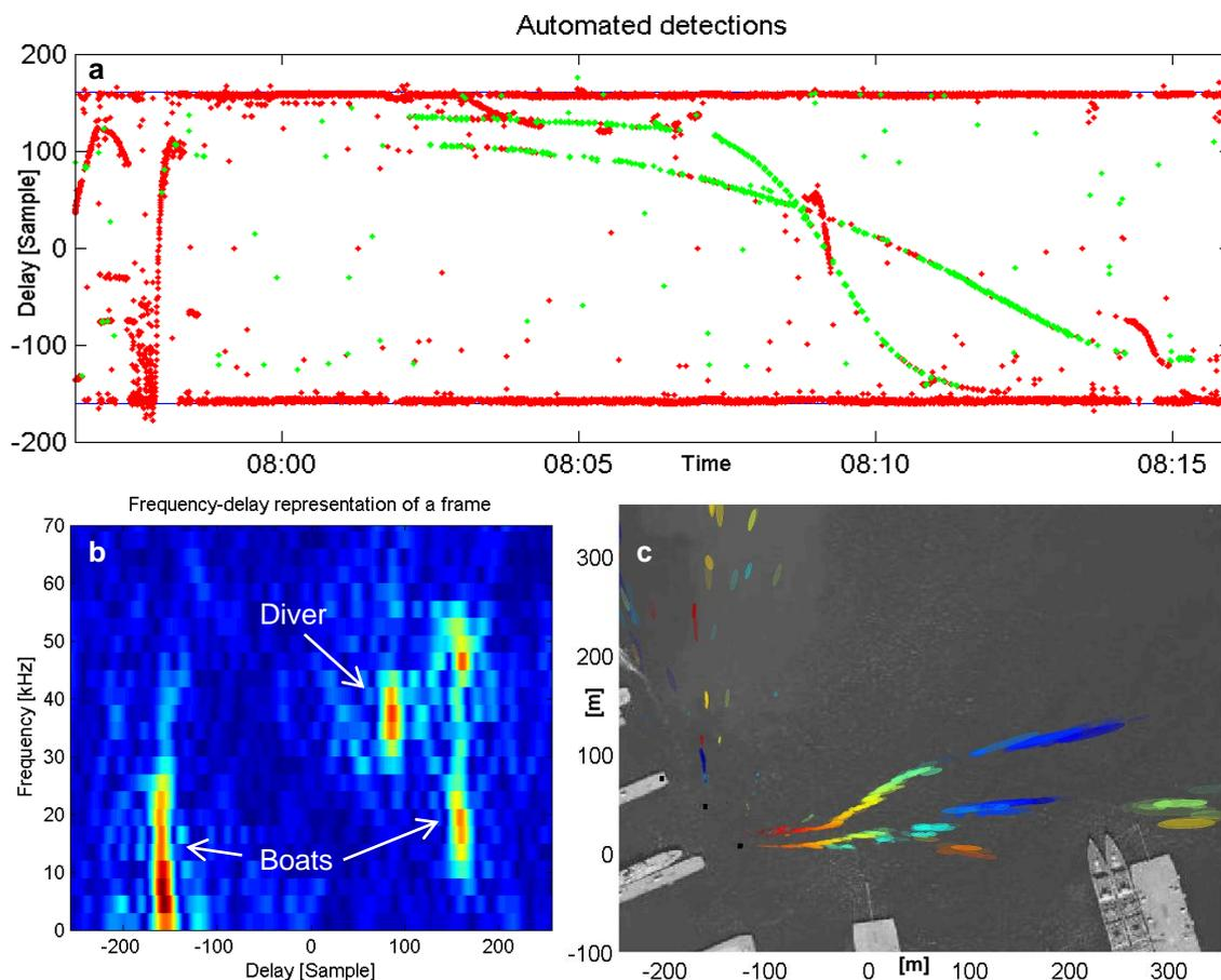
Fig.2: (a) Delays automatically detected in the correlation, color indicate frequency content (HF: red, LF: green). (b) Frequency-delay representation of a frame. (c) Localization obtained by combining the detections from three nodes (black squares). A localized target is represented by an ellipse located at the estimated target position. Its size represents the localization uncertainty and its color the time of detection (from blue to red). The two rainbow tracks correspond to divers.
