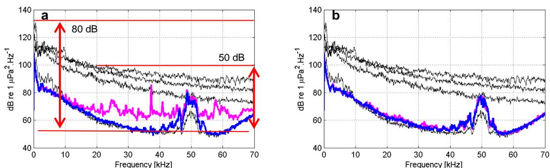
*Fig.3: Measured signal dynamic. The thin lines represent the power spectral density in the quietest and loudest conditions encountered during the trial. The thick lines represent the power spectral density during an automatically detected inhalation and just before it for a detection with good SNR (a) and a detection with low SNR (b). The detection shown in (b) is indicated by an arrow in Fig. 1d.*
