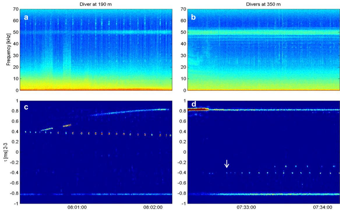
*Fig. 1: Spectrogram (a,b) and associated correlogram (c,d). Divers (dotted tracks) and boats (continuous tracks) are present in both cases. Diver's breathing is clearly visible in the spectrogram with the diver at 190 m but hardly visible with the divers at 350 m.*
