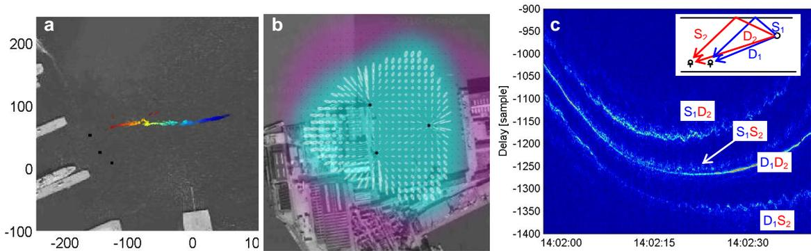
Fig.4: (a) Example of localization of a boat. (b) Illustration of sensor performance prediction (detection range). (c) Detail of a correlogram presenting the direct path and surface interactions.
