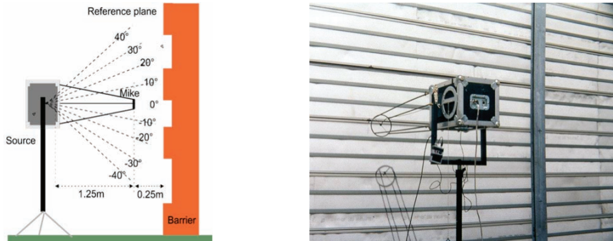
Figure 13: principles and application of the “ADRIENNE” method (CEN TS 1793-5)
