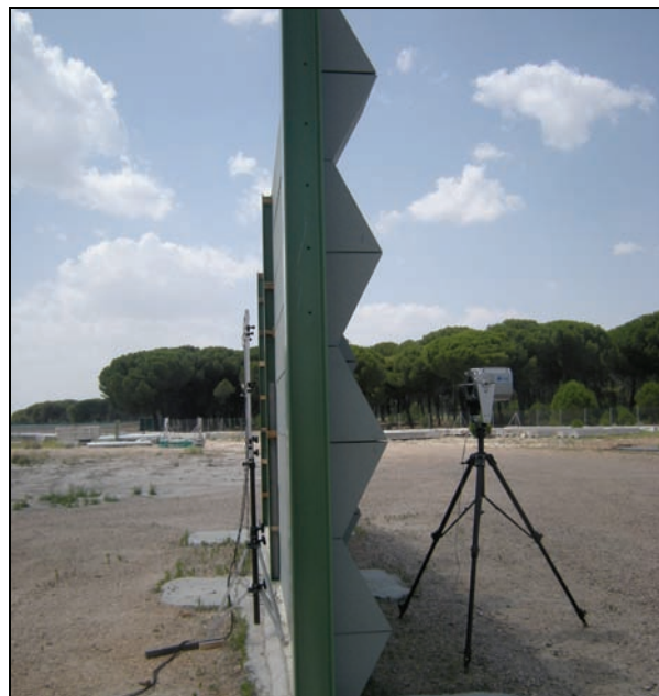
Figure 23: Left: sound reflection measurement in situ Right: measurement results in \frac{1}{3}^{\text{rd}} octave bands. DL_{RI} = 8 \text{ dB}
