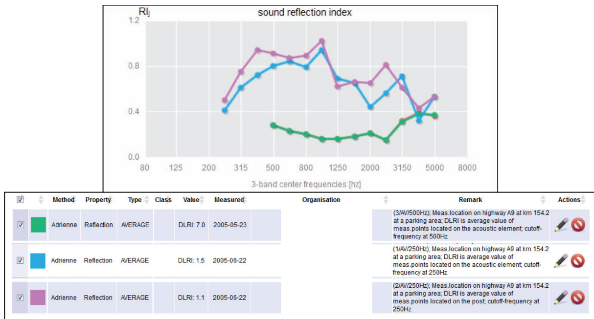
Figure 39: 1/3rd octave band results of sound reflection index according to CEN/TS 1793-5 The frequency in the remark field indicates the used lower cut-off frequency for the test
