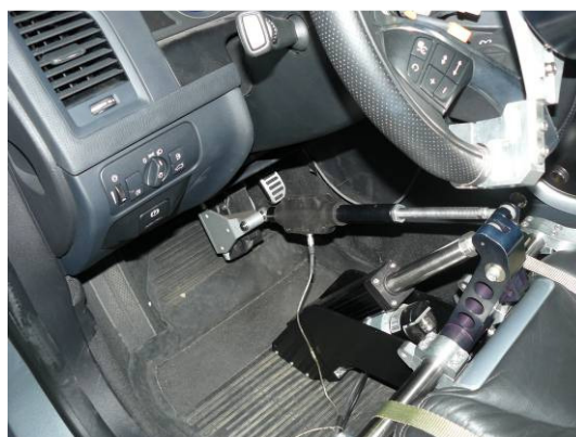
Braking robot installation
