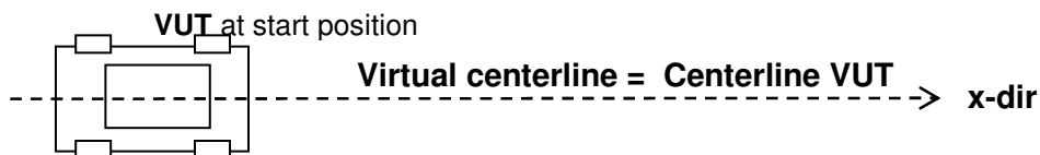
Figure 2-10-1: virtual centreline of the test as elongation of the VUT centreline at the beginning of the test
