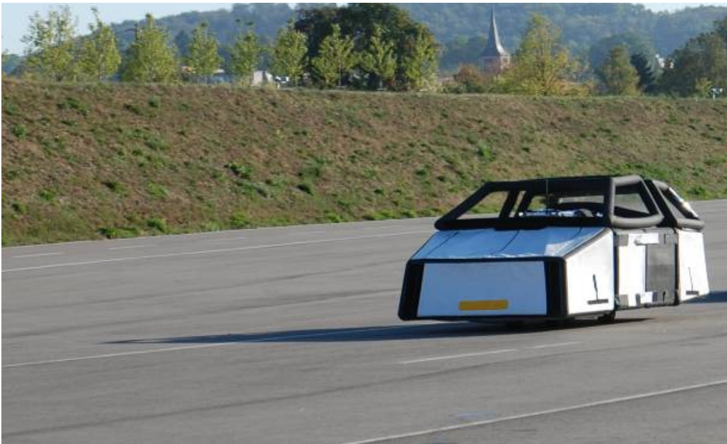
Figure 2-5 Mercedes test set up with AB Dynamics drive box
