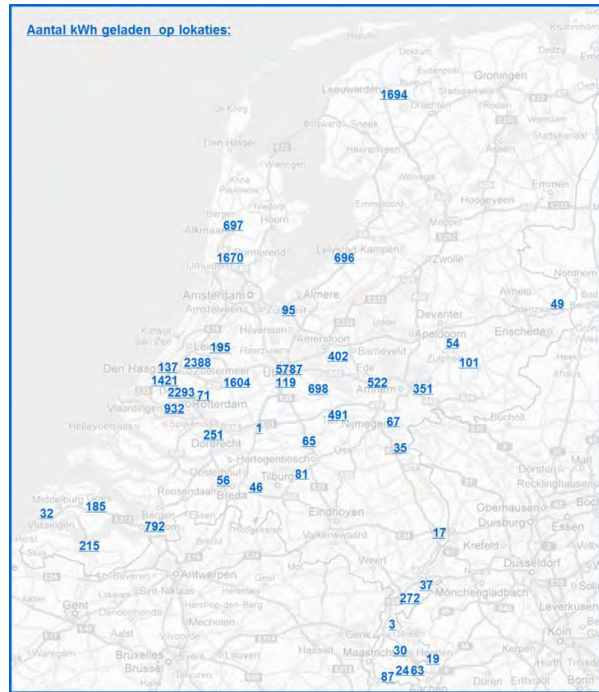
Figure 4 Overview of locations where the electric cars were charged during the field test. The amount of electrical energy charged at the location is shown in kilowatt hours (kWh).
