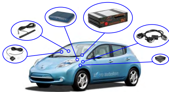
Figure 1 Metrics incorporated in each electric vehicle involved in the field test (from left to right): GPS antenna, GPRS antenna, GPRS unit, data logger, vehicle communication interface, on/off data logger module
