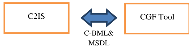
Figure 1. Data exchange between a C2IS and a CGF tool capable of C-BML & MSDL
