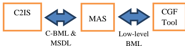
Figure 2 . Data exchange between a C2IS and a CGF tool using MAS
