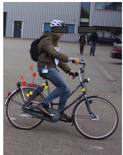
Figure 10: Definition of the coordinate system of the X-sens.
