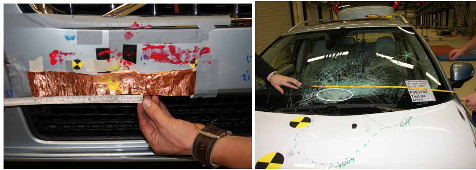
Figure 25: The color markings for the initial impact point of the bicycle and dummy
