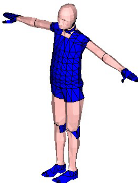
Figure 9. TNO 50 th percentile male occupant model as released with MADYMO v7.2
