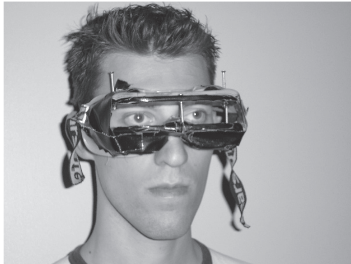
Figure 2.5: Participant wearing the modified pair of goggles providing a horizontal angular FoV size of 120°.
